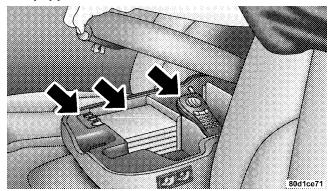
The center portion of the seat folds down to provide an armrest with unique storage compartments under the lid. Push the button on the front of the armrest to raise the cover. Inside there is a power outlet (if equipped),
